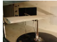
NREL S809 airfoil in University of Arizona wind tunnel. The model is equipped with 2 rows of pulsed vortex generator jets.
