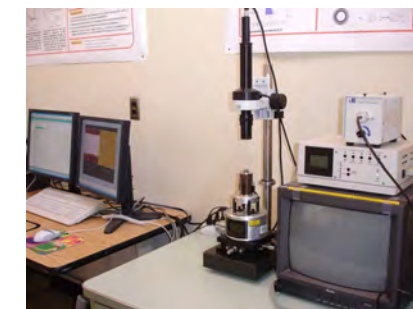
With the atomic force microscope in MGE we can analyze the impact of contaminants in municipal effluent on mineral recovery
