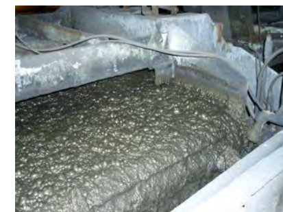
Flotation of chalcopyrite uses 16,800 gal/min of water at one mine
