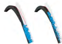
Simulations at Re=25,000. Instantaneous flow visualizations for uncontrolled "natural" flow (left) and controlled flow using pulsed vortex generator jets (right).
