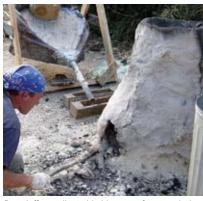
Dan Jeffery adjusts his bloomery furnace during an experiment to produce iron using an ancient technology.
