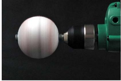
Professor A. Terry Bahill attached baseballs to an electric drill to simulate the patterns that result from various pitches. The two-seam fastball, shown here, is given away by its vertical red stripes.
