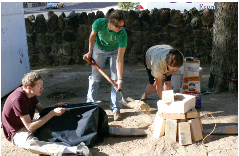
John Anesi, an anthropology sophomore, uses a hand-operated bellows to stoke the fire while Lesley Frame (center), a graduate student in materials science and engineering, adds sand to further insulate a crucible for melting copper. They were working on a demonstration experiment in Bronze Age technology during Materials Science of Art and Archaeological Objects, a Tier II science class taught by Pamela Vandiver (right).
